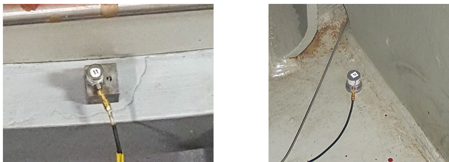
Figure 5.2. Accelerometers installed inside the ship, on the structure.
