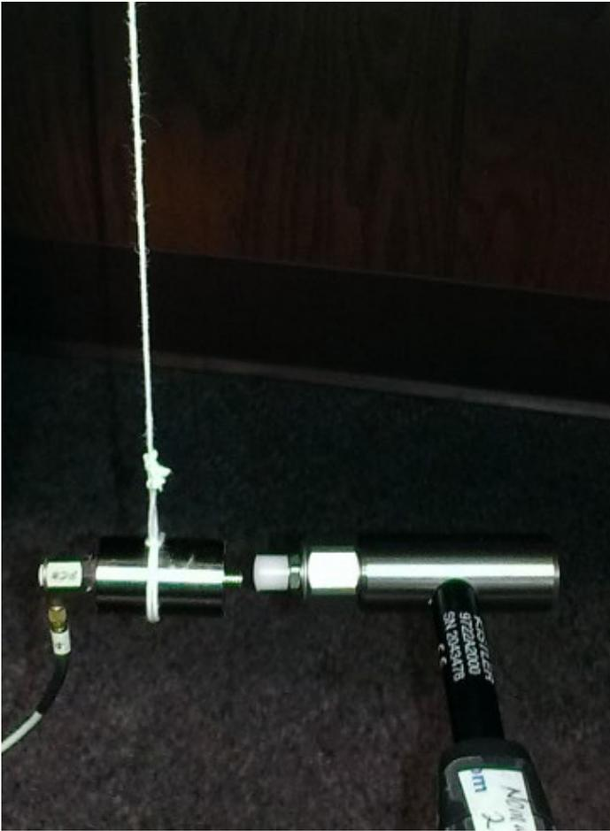
Figure 2: Improvised system to calibrate an impact hammer
