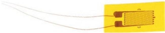
Figure 1: A strain gauge
