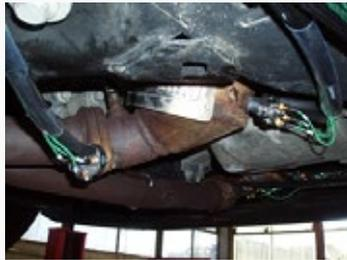
Supplied with cooling water via a windscreen washer pump, the accelerometer cables and cooling pipes were protected by over braiding to avoid damage under the vehicles during road tests, these were routed back to the instrumentation and pump/ water supply within the vehicles trunk/boot.
