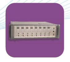
The LHP Filter is a modular switchable high or low pass filter unit available as a one channel DC powered unit or up to 8 channels in a AC/DC powered chassis. The units both use simple BNC input/output connectors on the front panel and offer user selectable AC/DC coupling as well as fixed IEPE signal source (4mA/24VDC) via a 3 way switch.
