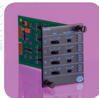
The V4/04 is a four channel QVC interface amplifier, providing a low cost, space efficient solution to multi channel piezotronic transducer interfacing at the expense of somewhat reduced flexibility. Each channel provides switched normalised outputs of 1 or 10g/V for transducer sensitivities of 10, 31.6, or 100mV/g. Gain is thus adjustable over the range x1 to x100 in 10dB increments.
