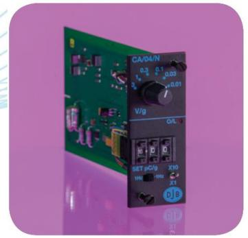
By way of example, with the amplifier normalised to 50pC/g a 10pC/g transducer rescales O/P1 to 2mV/g peak O/P1 level will increase from 1200 to 6000g ( $V_s = \pm 15V$ ).
