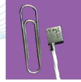
An Ultra-lightweight miniature triaxial vibration transducer comprising of three charge output piezo-electric accelerometer elements mounted orthogonally within a stainless steel block. It makes use of the independent shear plate sensing elements, ensuring a rugged and repeatable triaxial measurement under the most extreme conditions. This design will outperform single element devices. The AT/08 uses high temperature piezo-ceramics as standard to ensure thermal stability.
