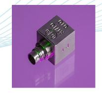
A lightweight miniature charge output triaxial vibration transducer with a single 4 pin connector, this is a unique design from DJB and comprises three charge output accelerometer piezo-electric elements mounted orthogonally within a titanium block. The use of the Konic Shear® independent sensing elements ensures a rugged and repeatable triaxial measurement under the most extreme conditions.
