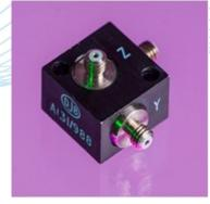
Lightweight triaxial vibration transducer compromising three Konic Shear® sensing elements all welded inserts bonded orthogonally into hard anodized aluminum housing.
