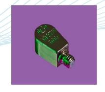
Sub-miniature teardrop charge output accelerometer. Manufactured in Titanium and features an all welded construction for a robust build. Using the DJB unique Konic shear® sensing element the low mass of the A/27/E renders it transparent in the vast majority of light weight structure vibration measurement applications.
