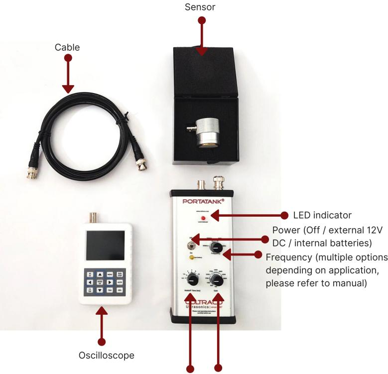
Holdoff Time (to control the period Gain (to increase incoming signal when the device starts to listen for strength to trigger LED indicator, the echo, please refer to manual)
